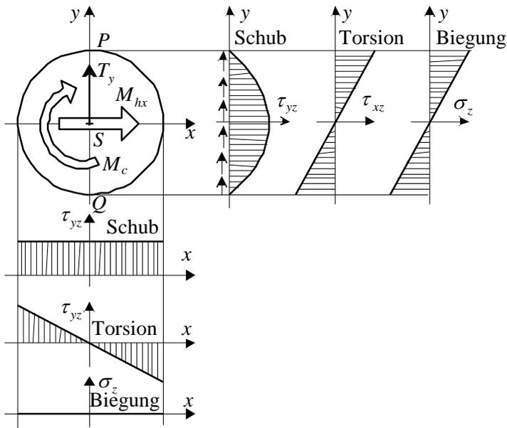
$$\tau_{yz} = -\frac{T_y S_x(y)}{I_x a(y)}, \quad \tau_{yz \max} = \frac{4T_y}{3A},$$
