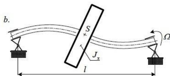
Vibration mode of the Laval rotor in the second critical rotational speed.
