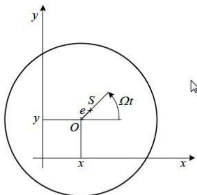
Disk of the Laval rotor. Point S is the center of gravity and point O is the geometrical center point of the rotor. The distance between point S and O is the eccentricity (e).
