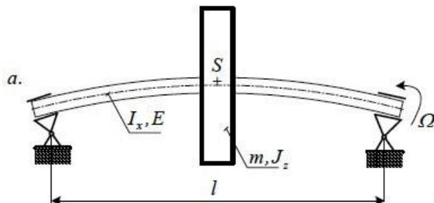
Vibration mode of the Laval rotor in the first critical rotational speed.
