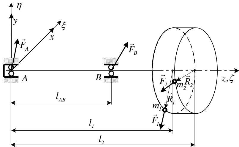
The  $\vec{F}_A$  bearing force and its  $\alpha$  angle between the vector and the  $x$  axis as well as  $\vec{F}_B$  bearing force and its  $\beta$  angle between the vector and the  $x$  axis are measured before balancing. The  $\alpha$  and  $\beta$  angles are in the  $xy$  plane.
