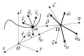
(30) What is the relationship between the absolute and relative acceleration of a point mass? Specify the meaning and calculation of the quantities in the relation.
