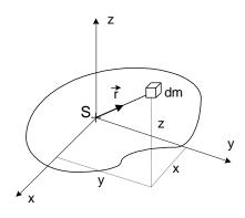
(50) Write down the tensor of moment of inertia about center of mass of a body with continuous mass distribution. What is its most important feature?
