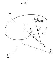
(49) Give an interpretation of the principal moments of inertia around axes x, y, z with respect to point S of a rigid body. Define the products of inertia.
