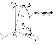
The most important feature is that the tangent vectors of a hodograph are the acceleration vectors.
